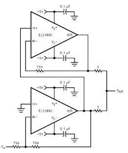
INVERTING 200mA OUTPUT CURRENT DISTRIBUTION AMPLIFIER
