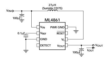
Figure 1. Application Test Circuit
