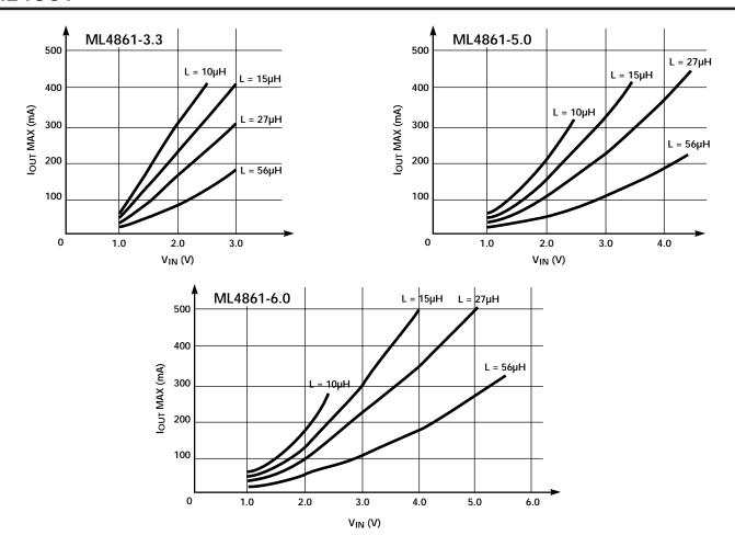
Figure 4. Output Current vs Input Voltage.
