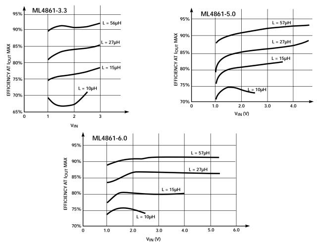
Figure 5. Typical Efficiency as a Function of V<sub>IN</sub>.
