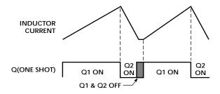
Figure 3. PFM Inductor Current Waveforms and Timing.
