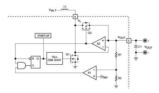
Figure 2. PFM Regulator Block Diagram
