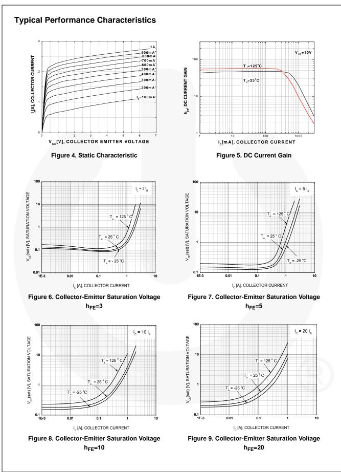
FJP2160D — ESBC<sup>™</sup> Rated NPN Silicon Transistor
