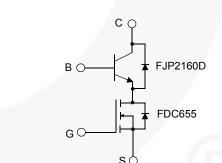
Figure 2. Internal Schematic Diagram Figure 3. ESBC Configuration<sup>(2)</sup>
