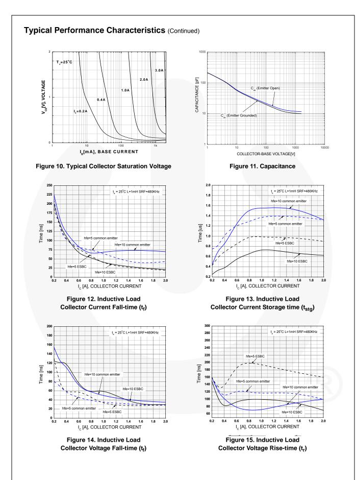
FJP2160D — ESBC<sup>™</sup> Rated NPN Silicon Transistor
