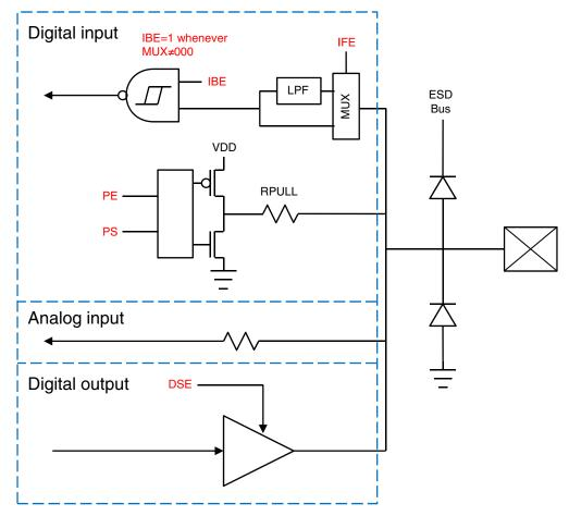
Figure 5. I/O simplified block diagram
