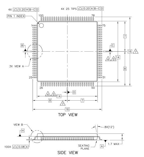
Figure 9. 100-pin LQFP package dimensions 1
