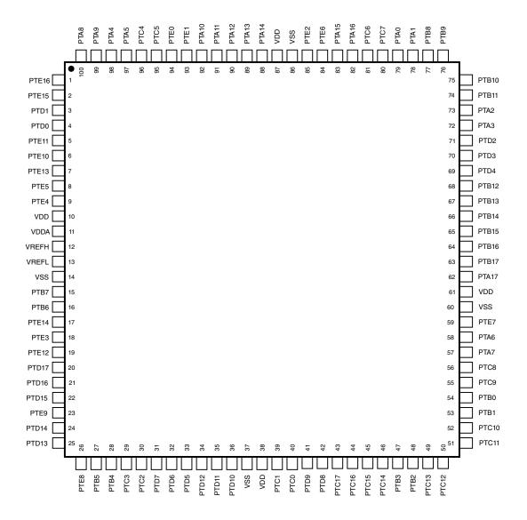
Figure 7. 100 LQFP Pinout Diagram
