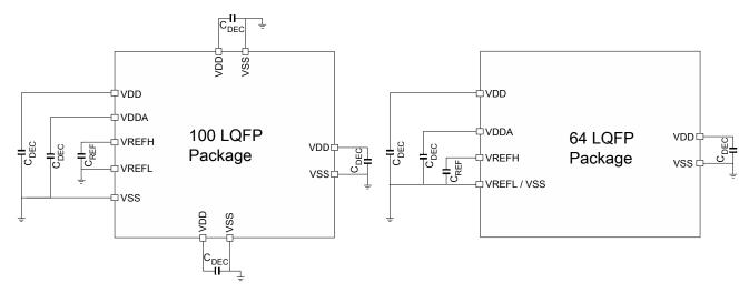
Figure 13. Pinout decoupling
