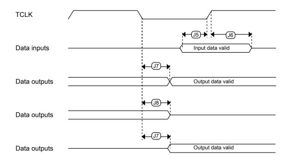
Figure 31. Boundary scan (JTAG) timing
