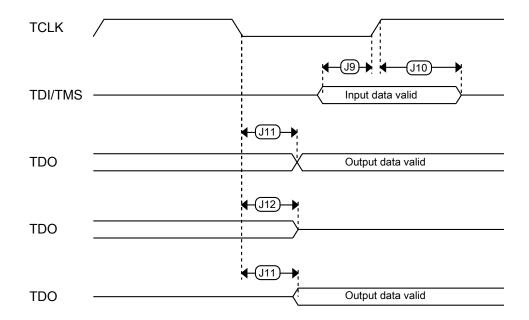
Figure 32. Test Access Port timing
