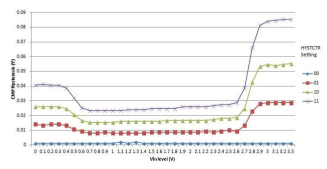
Figure 20. Typical hysteresis vs. Vin level (VDD = 3.3 V, PMODE = 0)
