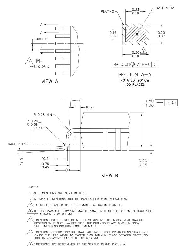
Figure 10. 100-pin LQFP package dimensions 2
