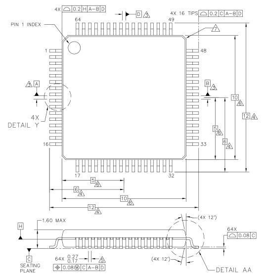
Figure 11. 64-pin LQFP package dimensions 1
