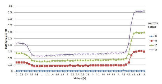
Figure 23. Typical hysteresis vs. Vin level (VDD = 5 V, PMODE = 1)
