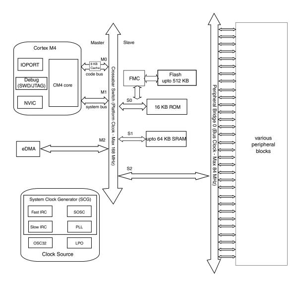
Figure 2. System diagram
