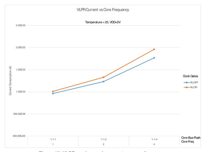
Figure 15. VLPR mode supply current vs. core frequency
