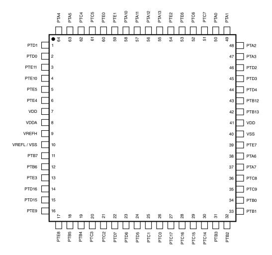
Figure 8. 64 LQFP Pinout Diagram
