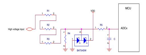
Figure 35. High voltage measurement with an ADC input
