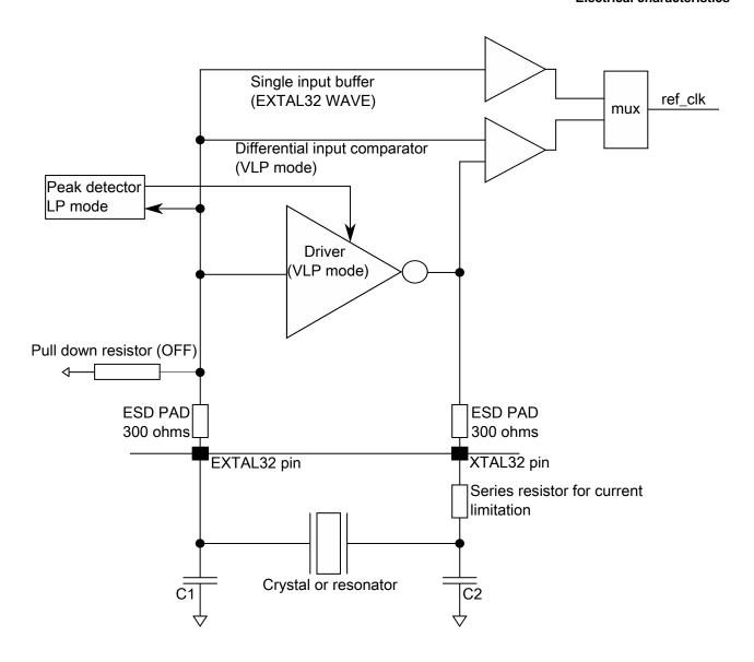
Figure 17. Oscillator connections scheme (OSC32)
