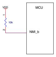
Figure 38. NMI pin biasing
