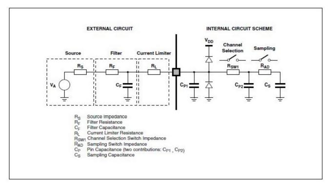
Figure 19. ADC input impedance equivalency diagram
