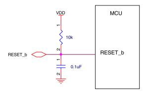
Figure 36. Reset circuit
