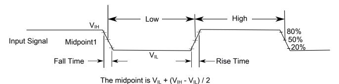
Figure 16. Input signal measurement reference
