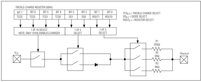
Figure 5. Programmable Trickle Charger
