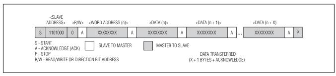
Figure 7. Data Write—Slave Receiver Mode
