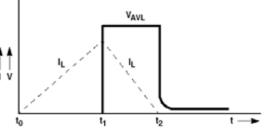
AVALANCHE CURRENT AND VOLTAGE WAVEFORMS
