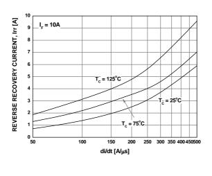
Figure 2. Typical Reverse Current
