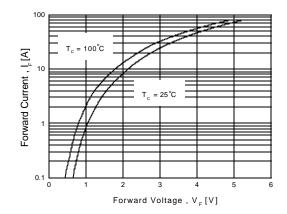
Figure 1. Typical Forward Voltage Drop vs. Forward Current
