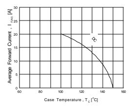
Figure 6. Forward Current Derating Curve
