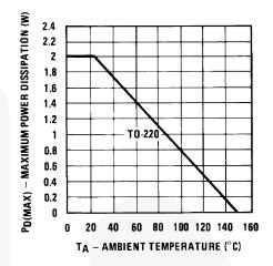
Figure 8. Maximum Power Dissipation vs. Ambient Temperature
