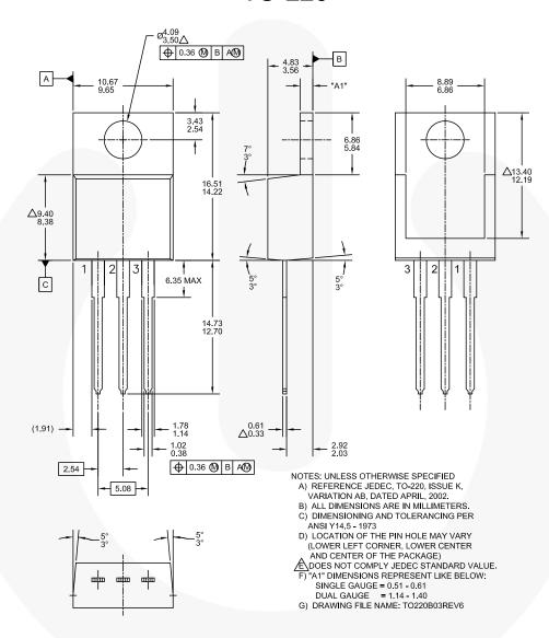
Figure 10. TO-220, MOLDED, 3-LEAD, JEDEC VARIATION AB (ACTIVE)
