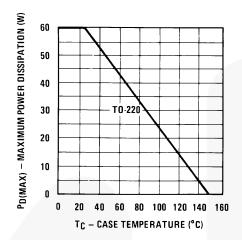
Figure 7. Maximum Power Dissipation vs. Case Temperature
