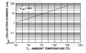
Figure 5. Collector Cut-Off Current vs.
