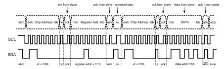
Figure 43. I<sup>2</sup>C Read Cycle
