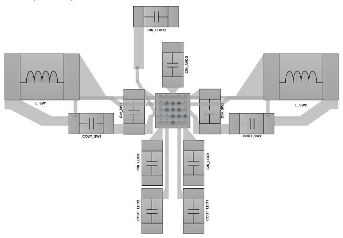
Figure 49. LP3907 DSBGA Layout Example
