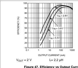
Figure 47. Efficiency vs Output Current (Forced PWM Mode)
