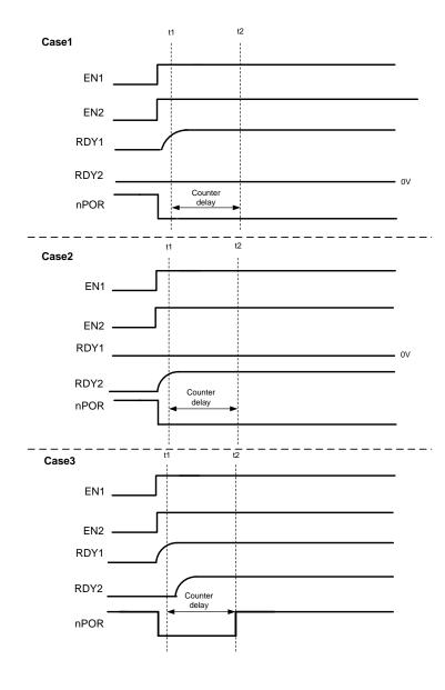
Figure 35. nPOR with Counter Delay
