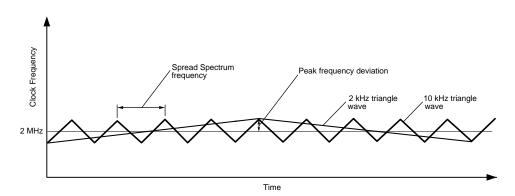
Figure 44. Spread Spectrum Modulation Frequency
