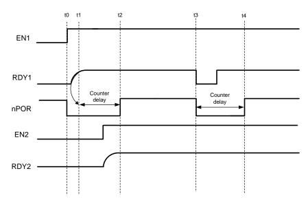
Figure 36. Faults Occurring in Counter Delay After Start-Up
