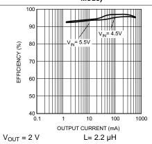
Figure 21. Efficiency vs Output Current (PWM-to-PFM Mode)
