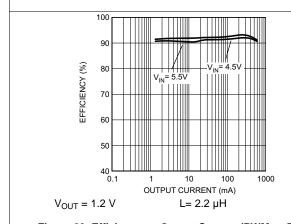
Figure 20. Efficiency vs Output Current (PWM-to-PFM Mode)
