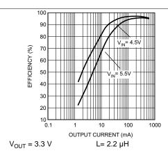
Figure 19. Efficiency vs Output Current (Forced PWM Mode)
