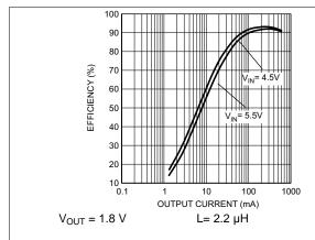
Figure 18. Efficiency vs Output Current (Forced PWM Mode)
