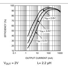
Figure 15. Efficiency vs Output Current (Forced PWM Mode)
