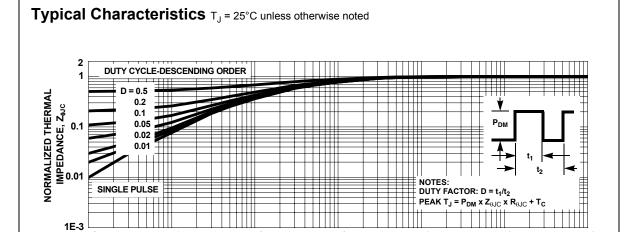
Figure 13. Transient Thermal Response Curve
