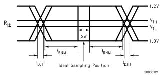
SW - Setup and Hold Time (Internal Data Sampling Window)  $t_{\text{DJIT}}$  - Serializer Output Bit Position Jitter that results from Jitter on TCLK  $t_{\text{RMM}}$  = Receiver Noise Margin Time
