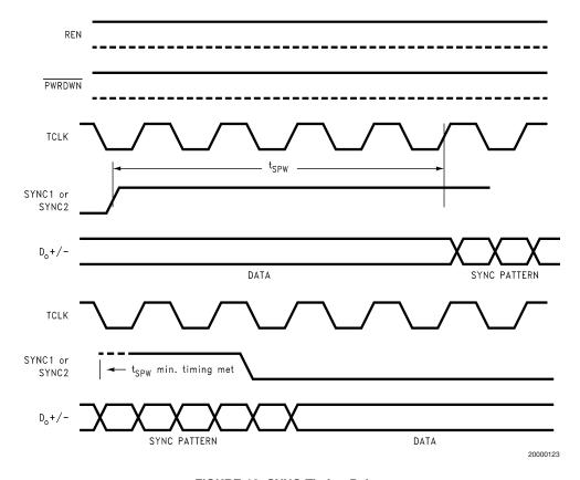
FIGURE 10. SYNC Timing Delays
