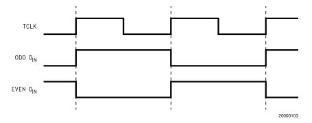
FIGURE 2. "Worst Case" Serializer ICC Test Pattern
