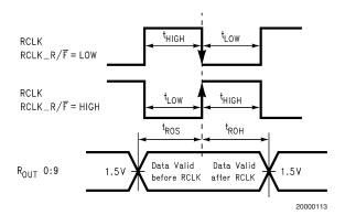
$\label{eq:timing_shown} \begin{aligned} & \text{Timing shown for RCLK\_R/$\overline{F}$ = LOW} \\ & \text{Duty Cycle } (t_{RDC}) = \underbrace{ t_{HIGH} \\ t_{HIGH} \ + \ t_{LOW} } \end{aligned}$
