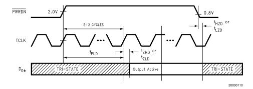
FIGURE 9. Serializer PLL Lock Time, and PWRDN TRI-STATE Delays
