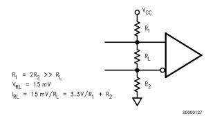
FIGURE 19. Failsafe Biasing Setup
