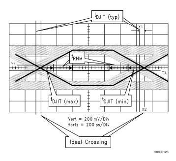
FIGURE 20. Using  $t_{\text{DJIT}}$  and  $t_{\text{RNM}}$  to Generate an Eye Pattern Mask and Validate Signal Quality
