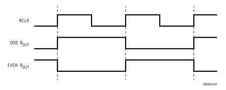
FIGURE 3. "Worst Case" Deserializer ICC Test Pattern
