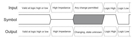
Figure 6.2 Input, Output, and Timing Reference Levels
