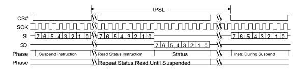
Figure 10.54 10.55 Program Resume (PGRS 8Ah) Command Sequence
