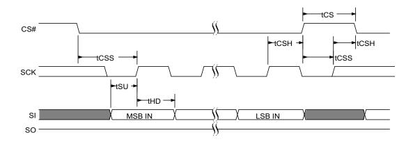
Figure 6.10 SPI Single Bit Output Timing
