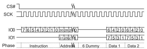
Figure 10.33 Dual I/O Read Command Sequence (4-Byte Address, BCh or BBh [ExtAdd=1], EHPLC=10b)
