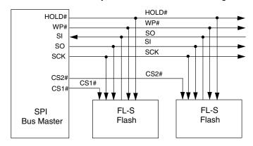
Figure 3.3 Bus Master and Memory Devices on the SPI Bus — Dual Bit Data Path
