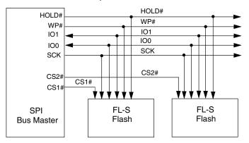
Figure 3.4 Bus Master and Memory Devices on the SPI Bus — Quad Bit Data Path
