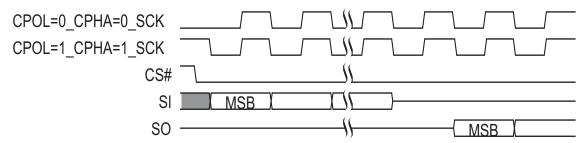
Timing diagrams throughout the remainder of the document are generally shown as both mode 0 and 3 by showing SCK as both high and low at the fall of CS#. In some cases a timing diagram may show only mode 0 with SCK low at the fall of CS#. In such a case, mode 3 timing simply means clock is high at the fall of CS# so no SCK rising edge set up or hold time to the falling edge of CS# is needed for mode 3.
