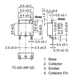
**Note** The depth of notch at the top of the fin is from 0 to 0.2 mm.
