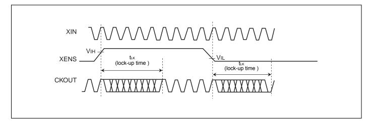
For modulation enable control using the XENS pin during normal operation, the set clock signal is output from CKOUT pin at most the lock-up time ( $t_{LK}$ ) after the level at the XENS pin is determined.
