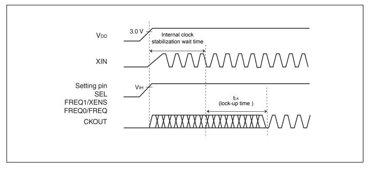
If the setting pin is fixed at the "H" or "L" level, the maximum time after the power is turned on until the set clock signal is output from CKOUT pin is (the stabilization wait time of input clock to XIN pin) + (the lock-up time " $t_{LK}$ "). For the input clock stabilization time, check the characteristics of the resonator or oscillator used.
