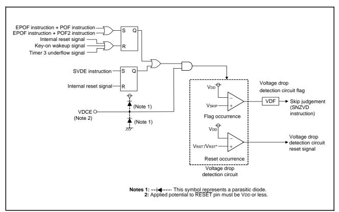
Fig 53. Voltage drop detection reset circuit
