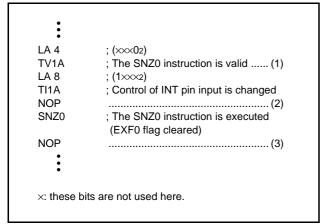
Fig 29. External 0 interrupt program example-1
