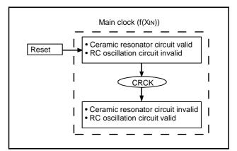
Fig 60. Switch to ceramic resonance/RC oscillation
