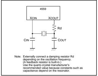
Fig 65. External quarts-crystal circuit
