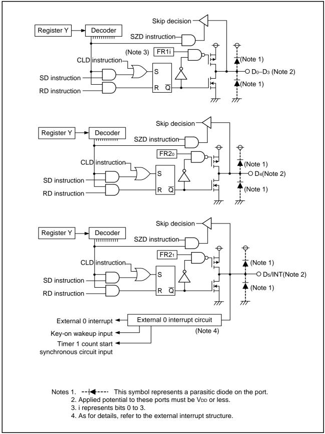
Fig 3. Port block diagram (1)
