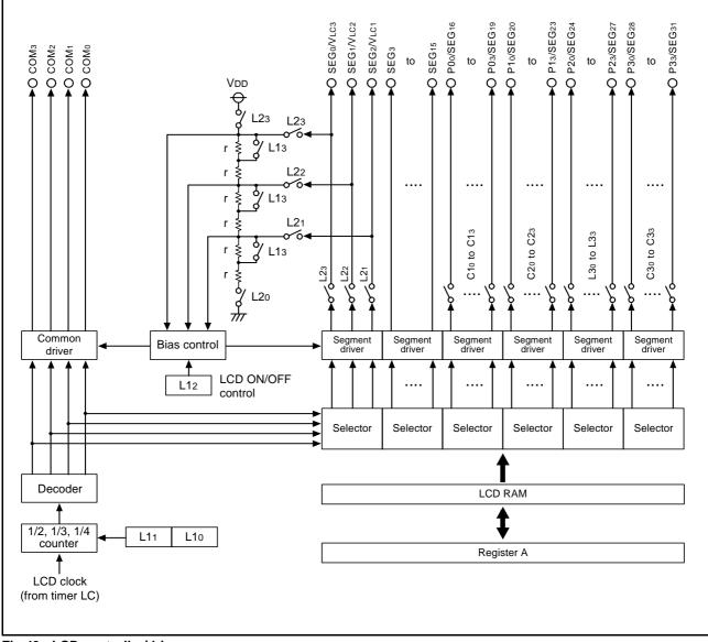
Fig 43. LCD controller/driver
