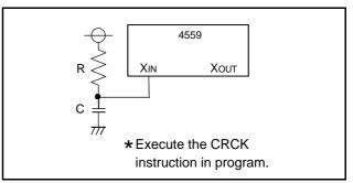
Fig 63. External RC oscillation circuit
