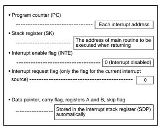
Fig 25. Internal state when interrupt occurs
