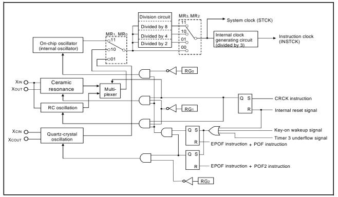
Fig 59. Clock control circuit structure
