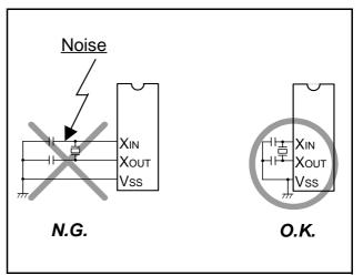
Fig 75. Wiring for clock I/O pins
