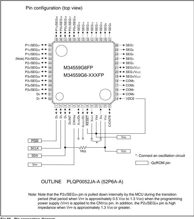
Fig 66. Pin connection diagram
