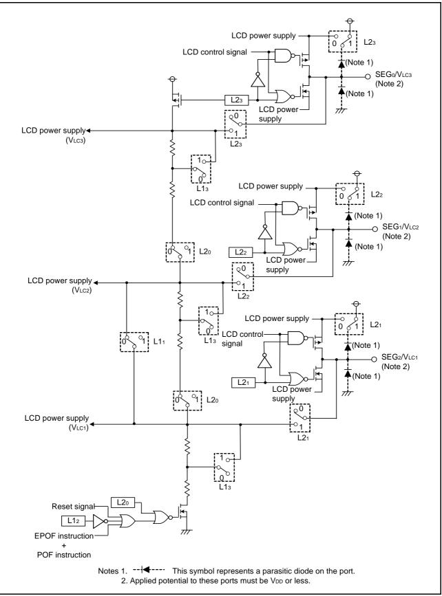
Fig 10. Port block diagram (8)
