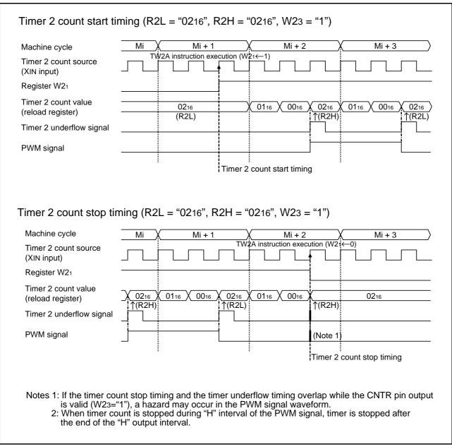
Fig 39. Timer count start/stop timing
