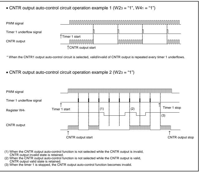
Fig 38. CNTR output auto-control function by timer 1
