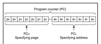
Fig 18. Program counter (PC) structure
