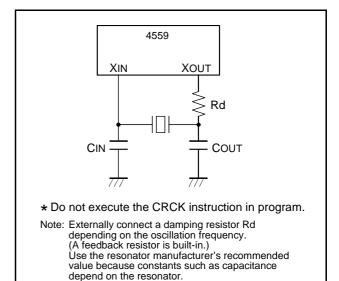
Fig 62. Ceramic resonator external circuit
