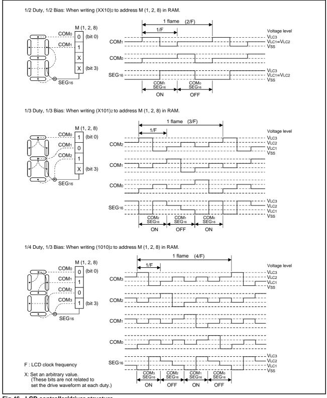
Fig 46. LCD controller/driver structure
