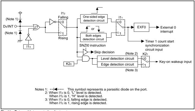
Fig 11. External interrupt circuit structure
