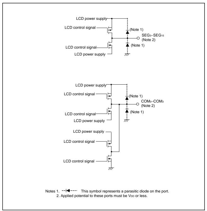
Fig 9. Port block diagram (7)
