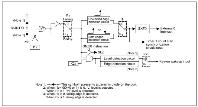
Fig 28. External interrupt circuit structure
