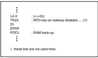
Fig 69. External 0 interrupt program example-2
