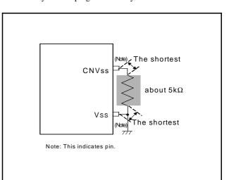
Fig 76. Wiring for CNVss pin
