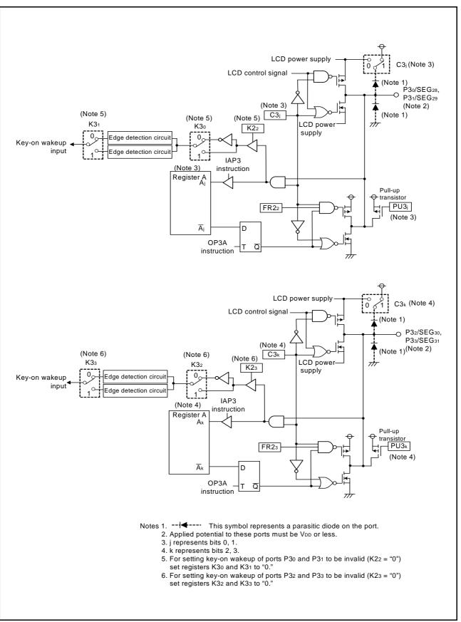
Fig 8. Port block diagram (6)
