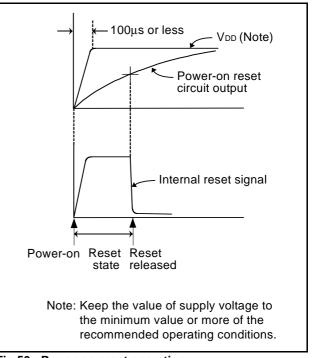
Fig 50. Power-on reset operation
