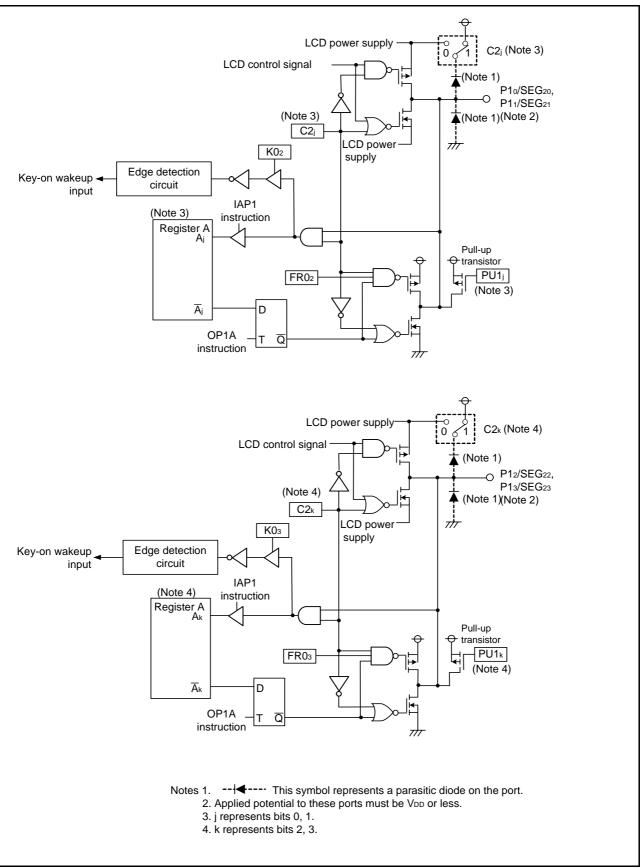
Fig 6. Port block diagram (4)
