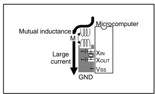
Fig 78. Wiring for a large current signal line
