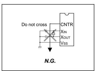
Fig 79. Wiring to a signal line where potential levels change frequently
