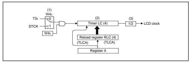
Fig 44. LCD clock control circuit structure
