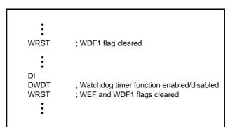
Fig 41. Program example to start/stop watchdog timer
