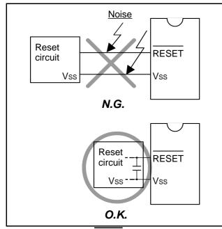
Fig 74. Wiring for the RESET input pin
