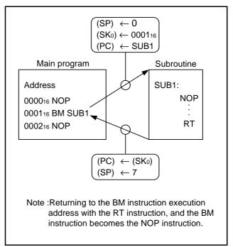
Fig 17. Example of operation at subroutine call
