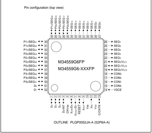
Fig 1. Pin configuration (PLQP0052JA-A type)
