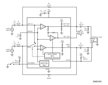
FIGURE 1. Typical Audio Amplifier Application Circuit
