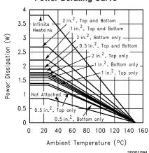
**Note 13:** This curve shows the LM4850LD's thermal dissipation ability at different ambient temperatures given the exposed-DAP of the part is soldered to a plane of 1oz. Cu with an area given in the label of each curve. This label also designated whether the plane exists on the same (top) layer as the chip, on the bottom layer, or on both layers. Infinite heatsink and unattached (no heatsink) conditions are also shown.
