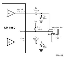
FIGURE 2. Headphone Control Circuit
