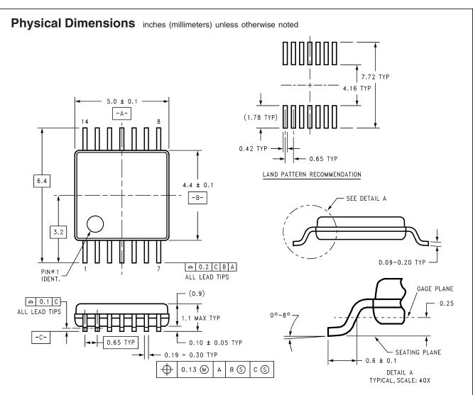
DIMENSIONS ARE IN MILLIMETERS MTC14 (REV C)
