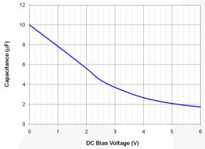
Figure 18. C<sub>EFF</sub> for 10 µF, 0402, X5R, 6.3 V-Rated Capacitor (TDK C1005X5R0J106M050BC)
