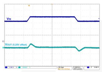
Figure 17. Line Transient, 3.2 <--> 3.9 V<sub>IN</sub>, 7  $\mu$ s Edge, 120 mA Load
