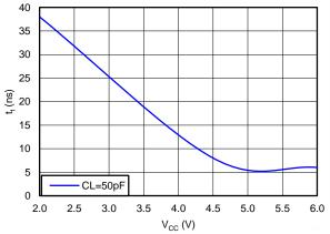
Figure 4. Transition Time vs V<sub>CC</sub>
