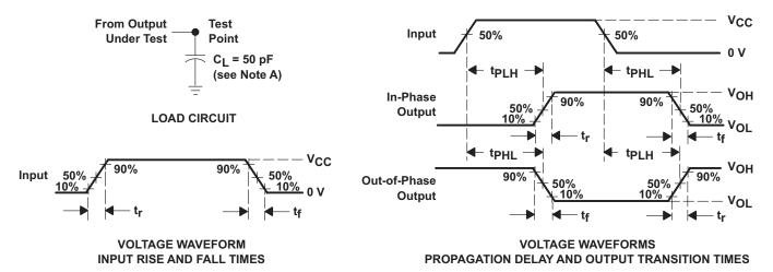
NOTES: A. CL includes probe and test-fixture capacitance.
