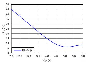
Figure 1. Propagation Delay vs V<sub>CC</sub>
