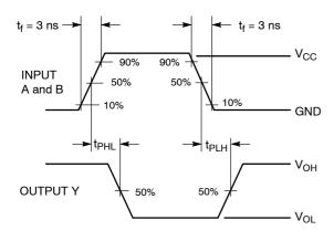
Figure 3. Switching Waveform
