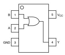
Figure 1. Pinout (Top View)
