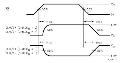
FIGURE 11. Driver TRI-STATE Waveforms
