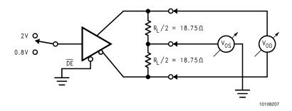
FIGURE 5. Differential Driver DC Test
