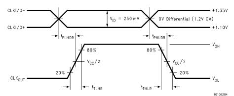
$Generator\ waveform\ for\ all\ test\ unless\ otherwise\ specified:\ f=25\ MHz,\ 50\%\ Duty\ Cycle,\ Zo=50\Omega,\ t_{TLH}=1\ ns,\ t_{THL}=1\ ns.$
