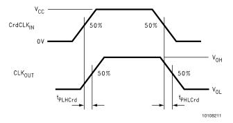
FIGURE 9.  $CrdCLK_{IN}$  Propagation Delay Time Waveforms
