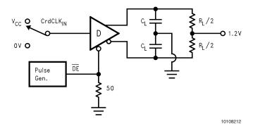
FIGURE 10. Driver TRI-STATE Test Circuit
