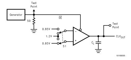
FIGURE 3. Output Enable (OE) Delay Test Circuit
