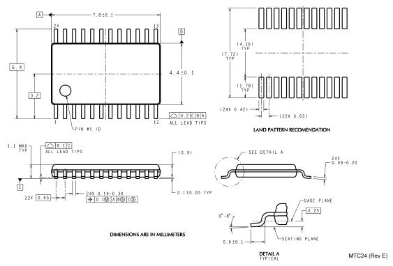
24-Pin TSSOP Package Drawing Dimensions shown in millimeters Order Number DS92CK16TMTC NS Package Number MTC24
