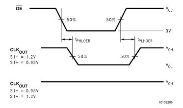
FIGURE 4. Output Enable (OE) Delay Waveforms
