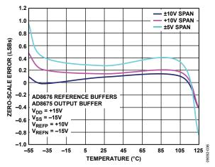
Figure 35. Zero-Scale Error vs. Temperature
