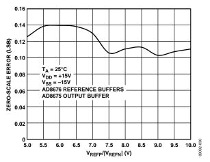
Figure 29. Zero-Scale Error vs. Reference Voltage
