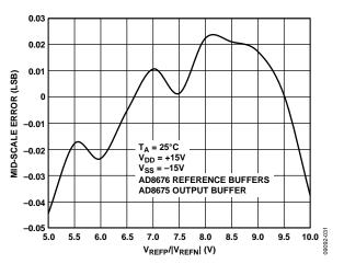
Figure 30. Midscale Error vs. Reference Voltage
