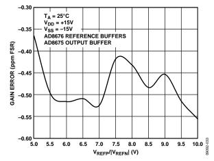
Figure 32. Gain Error vs. Reference Voltage
