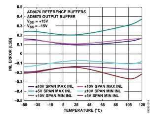
${\it Figure~13.}\ Integral~Nonlinear ity~Error~vs.~Temperature$
