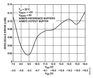
Figure 20. Zero-Scale Error vs. Supply Voltage, +5 V Span
