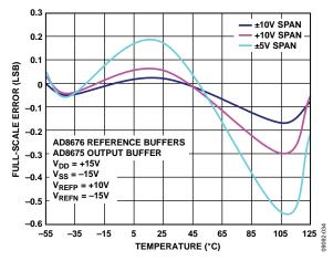
Figure 33. Full-Scale Error vs. Temperature
