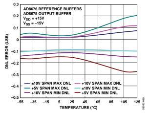
Figure 14. Differential Nonlinearity Error vs. Temperature
