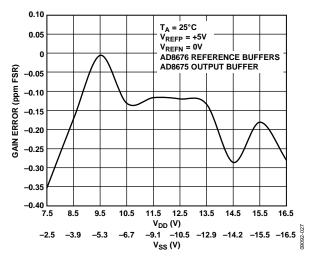
Figure 26. Gain Error vs. Supply Voltage, +5 V Span
