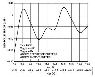
Figure 22. Midscale Error vs. Supply Voltage, +5 V Span
