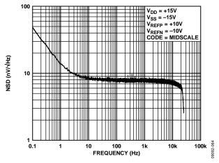
Figure 47. Noise Spectral Density vs. Frequency
