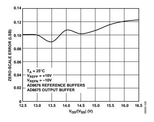
Figure 19. Zero-Scale Error vs. Supply Voltage, ±10 V Span
