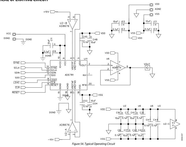
Figure 54 shows a typical operating circuit for the AD5781 using an AD8676 for reference buffers and an AD8675 as an output buffer. To meet the specified linearity, force sense buffers must be used on the reference inputs. Because the output impedance of the AD5781 is  $3.4\ k\Omega,$  an output buffer is required for driving low resistive, high capacitive loads.
