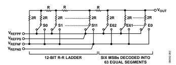
Figure 49. DAC Ladder Structure Serial Interface
