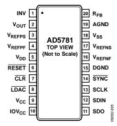
Figure 4. Pin Configuration
