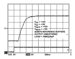
Figure 39. Rising Full-Scale Voltage Step
