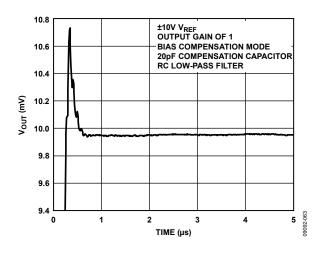
Figure 41. 125 Code Step Settling Time
