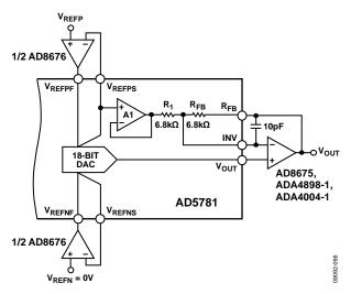
Figure 53. Output Amplifier in Gain of Two Configuration
