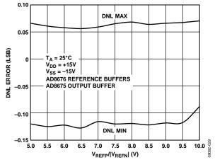
Figure 28. Differential Nonlinearity Error vs. Reference Voltage
