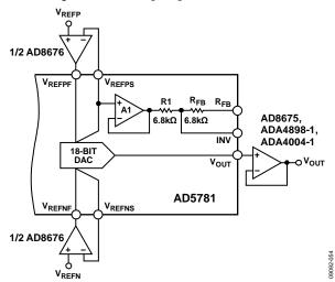
Figure 51. Output Amplifier in Unity Gain Configuration
