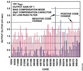
Figure 43. 6 MSB Segment Glitch Energy for 10 V V<sub>REF</sub>
