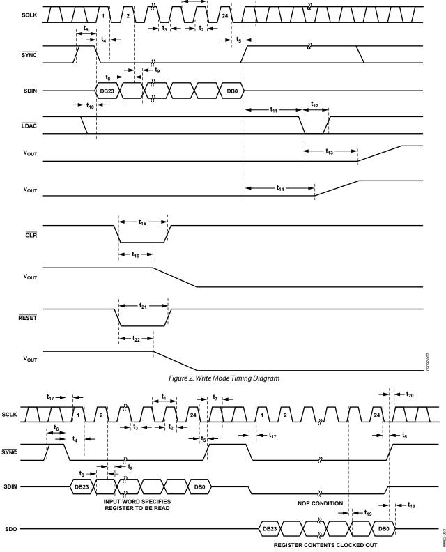
Figure 3. Readback Mode Timing Diagram
