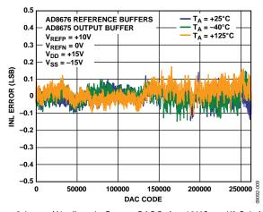
Figure 8. Integral Nonlinearity Error vs. DAC Code, ±10 V Span, X2 Gain Mode
