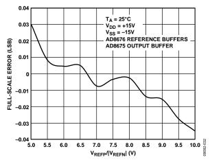
Figure 31. Full-Scale Error vs. Reference Voltage
