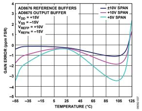
Figure 36. Gain Error vs. Temperature
