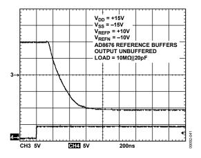
Figure 40. Falling Full-Scale Voltage Step
