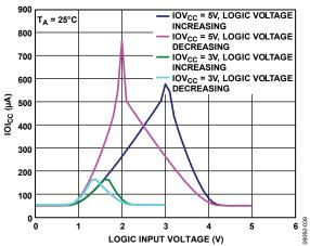
Figure 37. IOIcc vs. Logic Input Voltage
