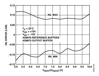
Figure 27. Integral Nonlinearity Error vs. Reference Voltage
