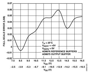
Figure 24. Full-Scale Error vs. Supply Voltage, +5 V Span
