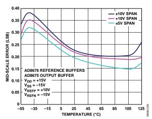
Figure 34. Midscale Error vs. Temperature
