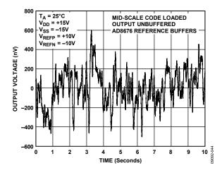
Figure 46. Voltage Output Noise, 0.1 Hz to 10 Hz Bandwidth
