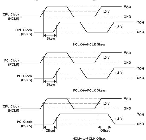
Figure 2. Waveforms for Calculation of t<sub>Skew</sub> and t<sub>offset</sub>
