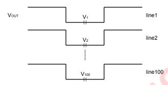
**Remark** This is measured by the DC level sampling of only the signal level, not by CDS (Correlated Double Sampling)
