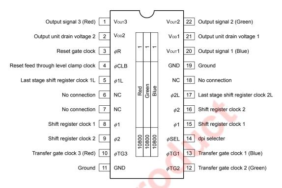
Caution Connect the no connection pins (NC) to GND.
