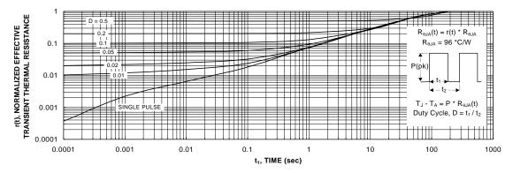
Figure 11. Transient Thermal Response Curve
