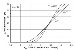
Figure 5. Transfer Characteristics
