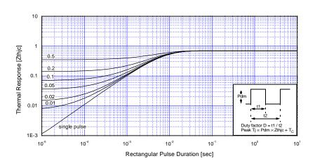
Fig 17. Transient Thermal Impedance of IGBT
