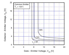
Fig 5. Saturation Voltage vs. V<sub>GE</sub>
