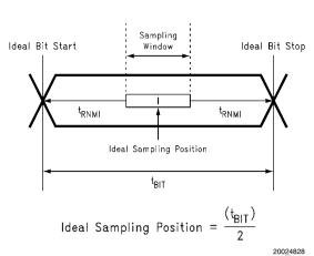
t<sub>RNMI-L</sub> is the ideal noise margin on the left of the figure, it is a negative value to indicate early with respect to ideal. t<sub>RNMI-R</sub> is the ideal noise margin on the right of the above figure, it is a positive value to indicate late with respect to ideal.
