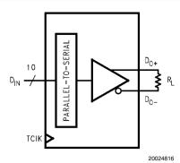
$V_{OD}$  = (DO+)–(DO<sup>-</sup>). Differential output signal is shown as (DO+)–(DO–), device in Data Transfer mode.
