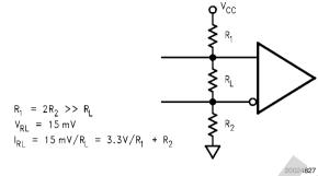
FIGURE 18. Failsafe Biasing Setup
