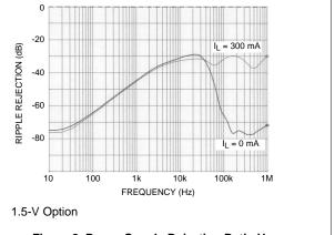
Figure 8. Power Supply Rejection Ratio  $V_{BATT}$
