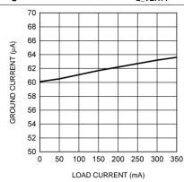
Figure 6. Ground Current vs Load Current
