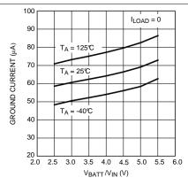
Figure 5. Ground Current vs  $V_{BATT} / V_{IN}$
