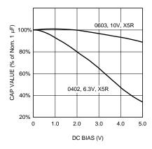
Figure 10. Typical Variation In Capacitance vs DC Bias
