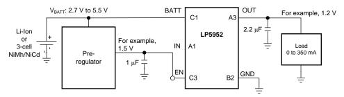
Figure 9. LP5952 Typical Application Circuit
