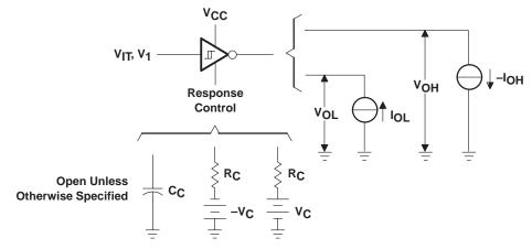
NOTE A: Arrows indicate actual direction of current flow. Current into a terminal is a positive value.
