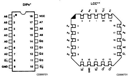
\*Also available in 18-pin Flatpack. Pinout identical to DIPs.
