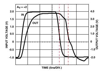
FIGURE 4. PULSE RESPONSE WITHOUT LIMITING
