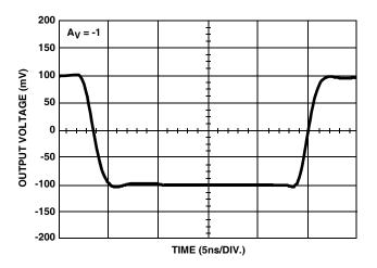
FIGURE 16. SMALL SIGNAL BIPOLAR PULSE RESPONSE
