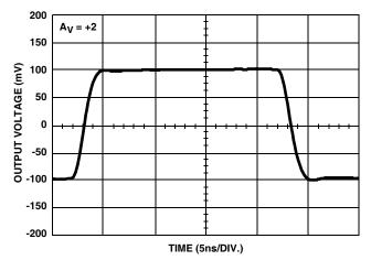
FIGURE 8. SMALL SIGNAL BIPOLAR PULSE RESPONSE
