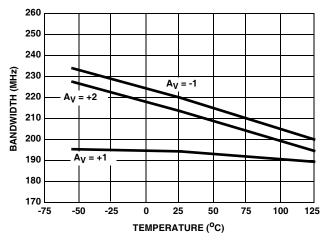
FIGURE 23. -3dB BANDWIDTH vs TEMPERATURE
