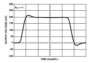
FIGURE 10. SMALL SIGNAL POSITIVE PULSE RESPONSE
