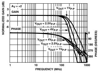
FIGURE 19. FREQUENCY RESPONSE FOR VARIOUS OUTPUT VOLTAGES
