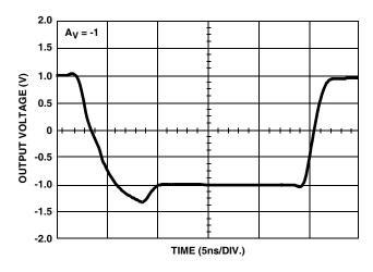
FIGURE 17. LARGE SIGNAL BIPOLAR PULSE RESPONSE
