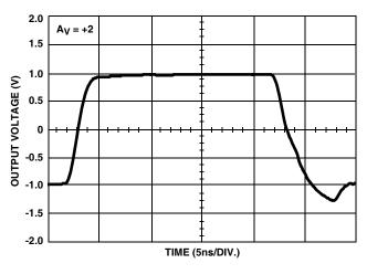
FIGURE 9. LARGE SIGNAL BIPOLAR PULSE RESPONSE
