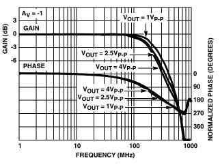
FIGURE 21. FREQUENCY RESPONSE FOR VARIOUS OUTPUT VOLTAGES
