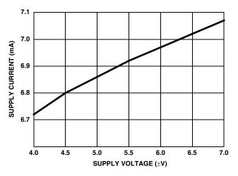
FIGURE 34. SUPPLY CURRENT vs SUPPLY VOLTAGE
