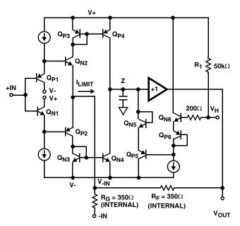
FIGURE 3. HFA1115 SIMPLIFIED VH LIMIT CIRCUITRY
