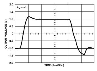
FIGURE 13. LARGE SIGNAL BIPOLAR PULSE RESPONSE
