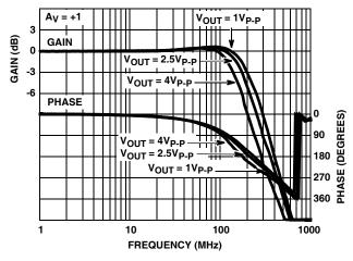
FIGURE 20. FREQUENCY RESPONSE FOR VARIOUS OUTPUT VOLTAGES
