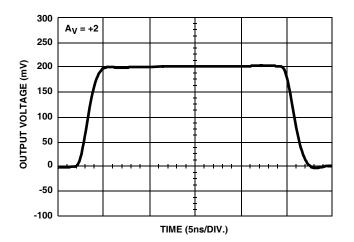
FIGURE 6. SMALL SIGNAL POSITIVE PULSE RESPONSE
