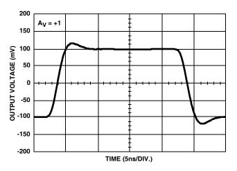
FIGURE 12. SMALL SIGNAL BIPOLAR PULSE RESPONSE
