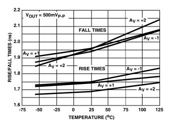
FIGURE 35. RISE AND FALL TIMES vs TEMPERATURE
