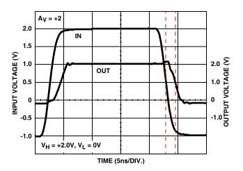
FIGURE 5. PULSE RESPONSE WITH LIMITING
