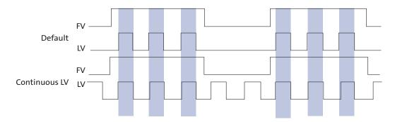
The timing of an entire frame is shown in Figure 10: "Line Timing and FRAME\_VALID/ LINE\_VALID Signals," on page 17.
