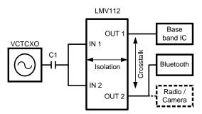
Figure 37. Isolation Block Diagram
