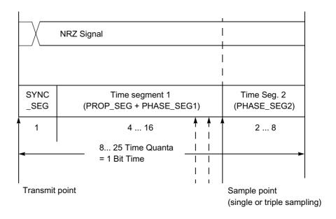
Figure 18-8. Segments within the Bit Time
