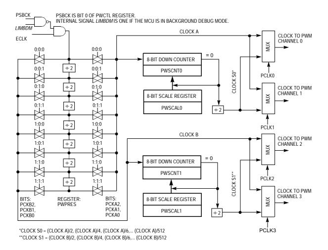
Figure 14-3. PWM Clock Sources
