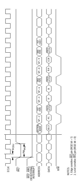
Figure 21-5. Interrupt Timing Diagram
