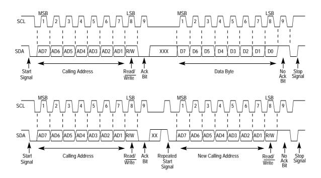
Figure 17-2. IIC Transmission Signals
