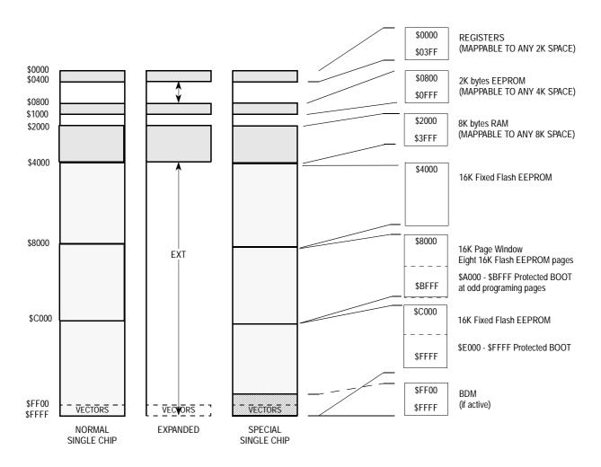
Figure 6-1. MC68HC912DT128A Memory Map after reset
