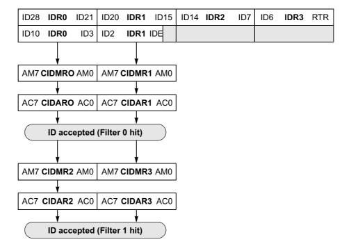
Figure 18-4. 16-bit Maskable Acceptance Filters
