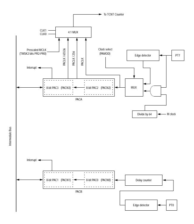
Figure 15-4. 16-Bit Pulse Accumulators Block Diagram
