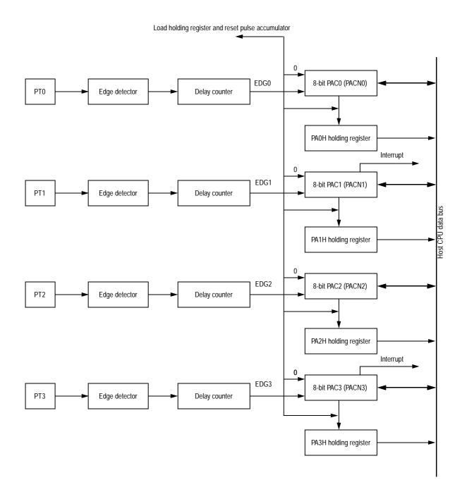
Figure 15-3. 8-Bit Pulse Accumulators Block Diagram
