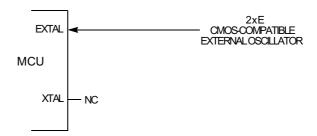
Figure 3-5. External Oscillator Connections
