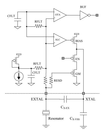
Figure 13-2. MC68HC912Dx128C Colpitts Oscillator Architecture
