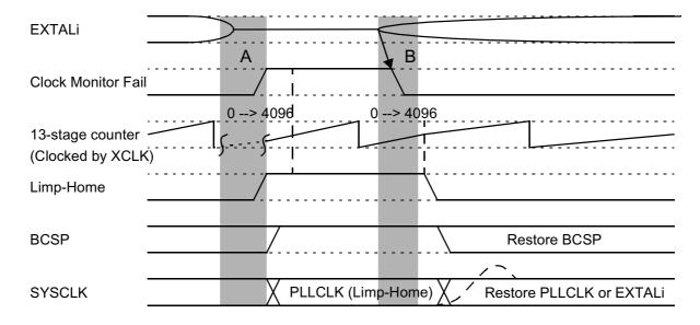
Figure 12-3. Clock Loss during Normal Operation
