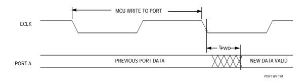
Figure 21-7. Port Write Timing Diagram
