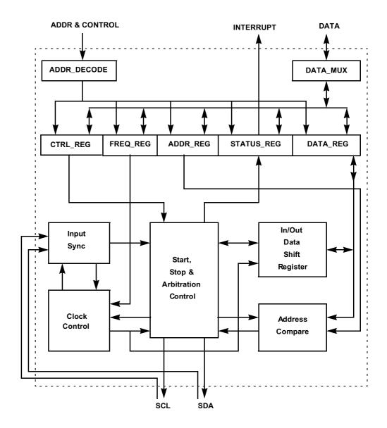
Figure 17-1. IIC Block Diagram
