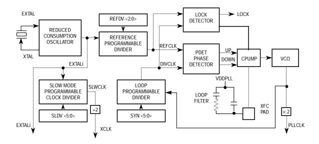
Figure 12-2. PLL Functional Diagram
