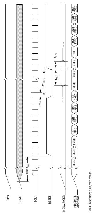
Figure 21-2. POR and External Reset Timing Diagram
