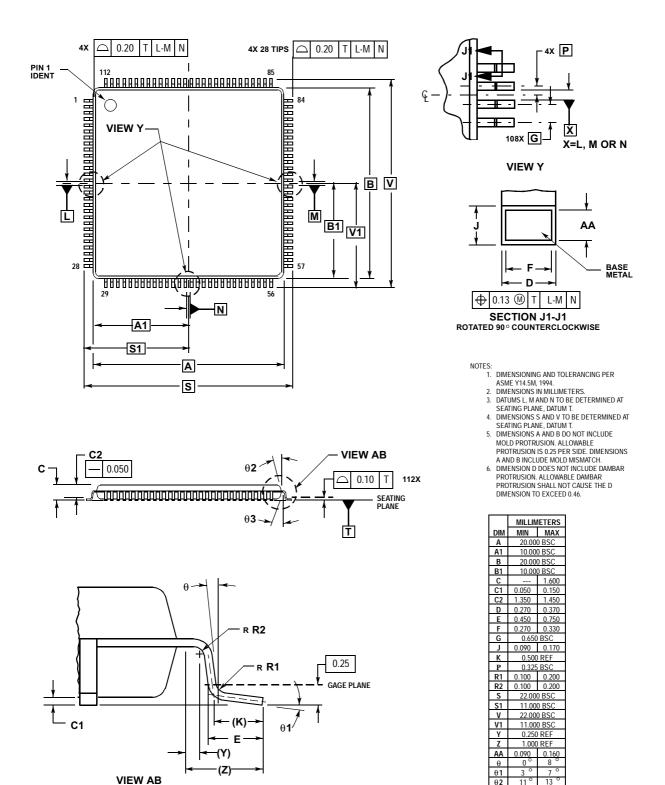
Figure 3-3. 112-pin QFP Mechanical Dimensions (case no. 987)
