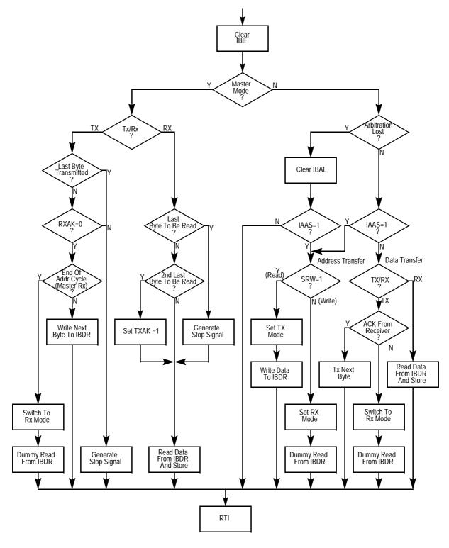
Figure 17-4. Flow-Chart of Typical IIC Interrupt Routine
