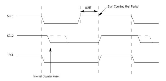
Figure 17-3. IIC Clock Synchronization
