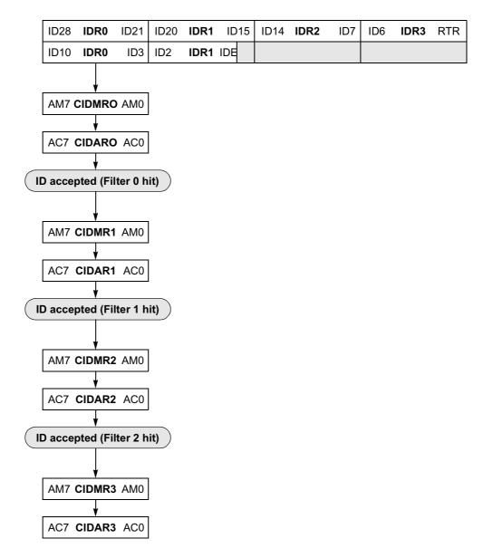
Figure 18-5. 8-bit Maskable Acceptance Filters
