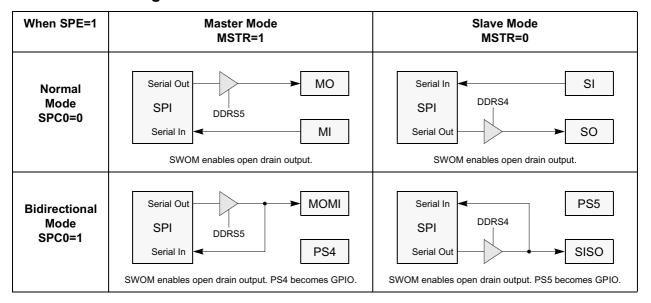
Figure 16-6. Normal Mode and Bidirectional Mode
