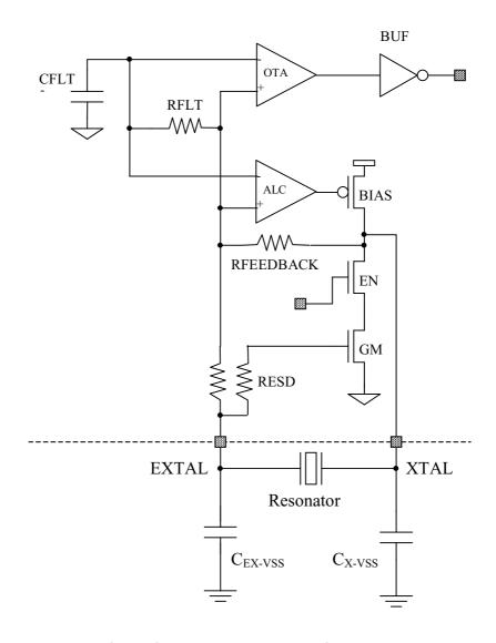
Figure 13-4. MC68HC912Dx128P Pierce Oscillator Architecture
