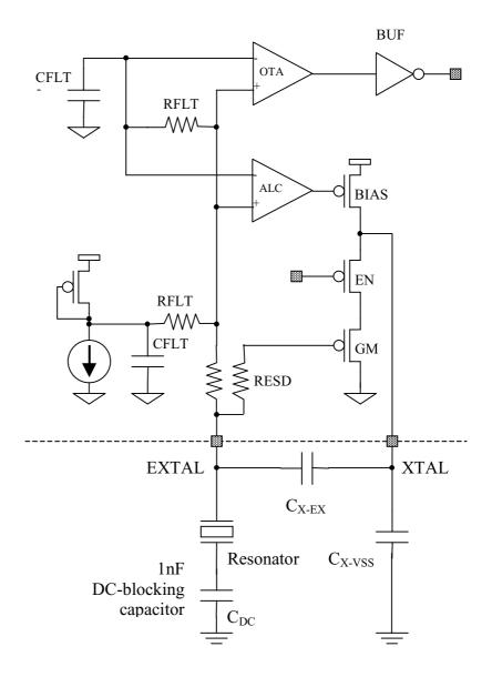
Figure 13-3. MC68HC912Dx128C Crystal with DC Blocking Capacitor
