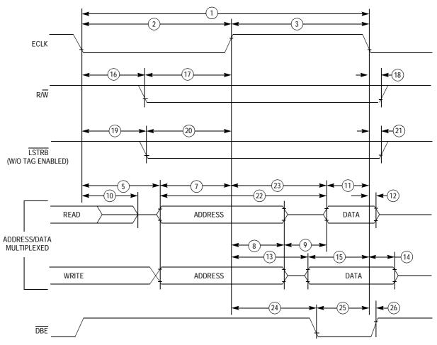
NOTE: Measurement points shown are 20% and 70% of  $V_{\mbox{\scriptsize DD}}$
