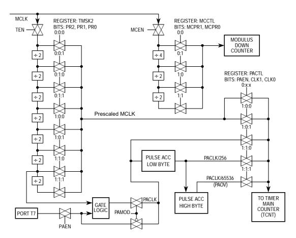
Figure 12-8. Clock Chain for ECT
