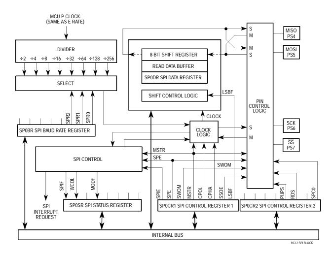
Figure 16-3. Serial Peripheral Interface Block Diagram
