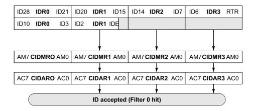
Figure 18-3. 32-bit Maskable Identifier Acceptance Filters
