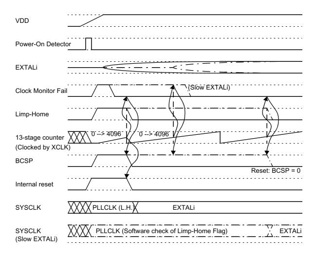
Figure 12-4. No Clock at Power-On Reset
