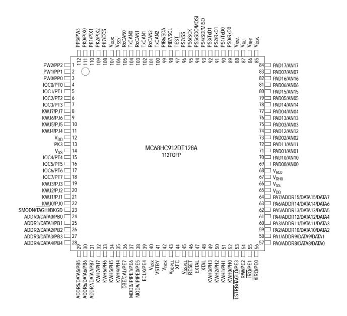
Note: TEST = This pin is used for factory test purposes. It is recommended that this pin is not connected in the application, but it may be bonded to 5.5 V max without issue.
