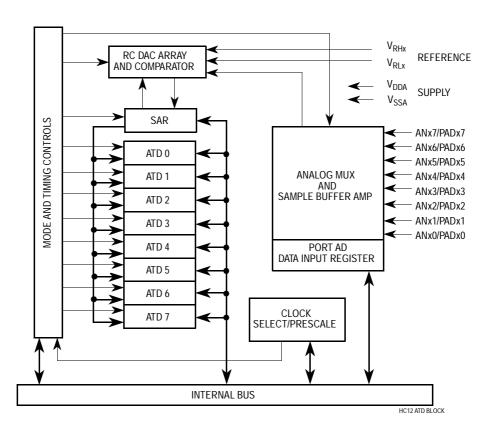
Figure 19-1. Analog-to-Digital Converter Block Diagram
