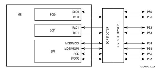
Figure 16-1. Multiple Serial Interface Block Diagram
