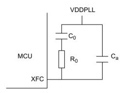
Figure 3-4. PLL Loop Filter Connections
