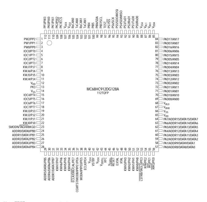
Note: TEST = This pin is used for factory test purposes. It is recommended that this pin is not connected in the application, but it may be bonded to 5.5 V max without issue.
