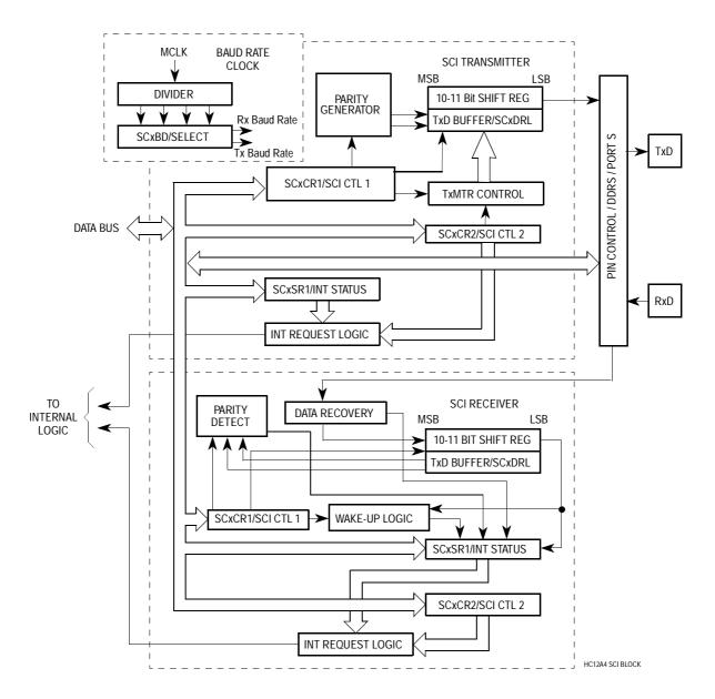
Figure 16-2. Serial Communications Interface Block Diagram
