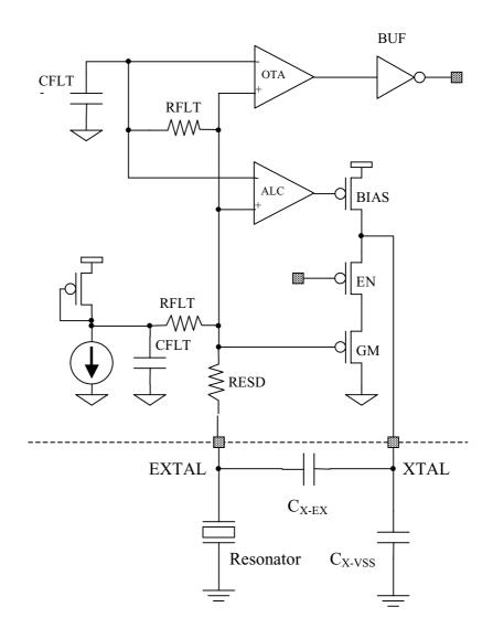
Figure 13-1. MC68HC912DT128A Colpitts Oscillator Architecture
