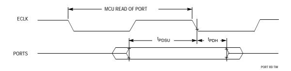
Figure 21-6. Port Read Timing Diagram
