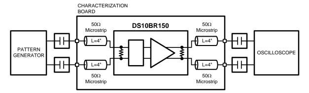
Figure 5. Jitter Measurements Test Circuit
