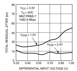
Figure 13. Total Jitter as a Function of Input Amplitude
