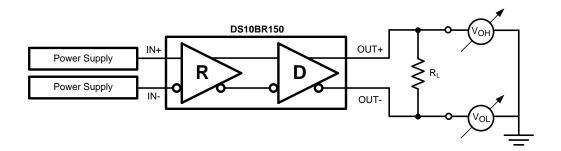
Figure 1. Differential Driver DC Test Circuit
