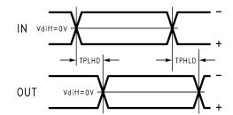
Figure 3. Propagation Delay Timing Diagram
