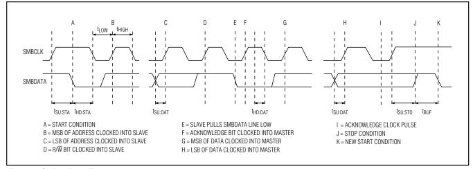
Figure 9. SMBus Read Timing
