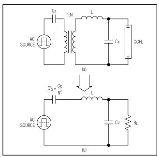
Figure 4. Equivalent Resonant Tank Circuit
