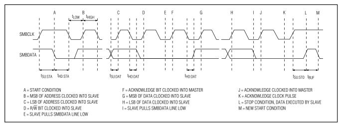
Figure 8. SMBus Write Timing
