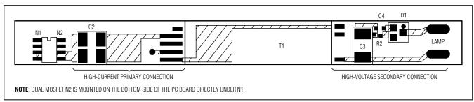
Figure 10. High-Voltage Components Layout Example
