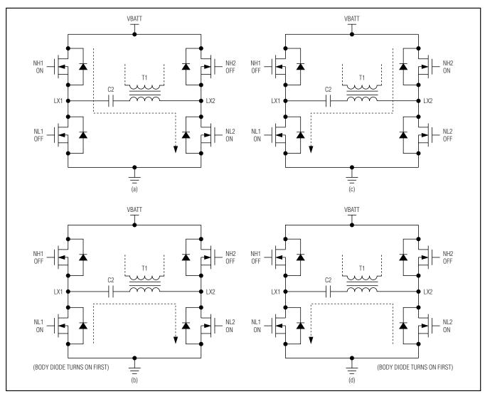
Figure 3. Resonant Operation
