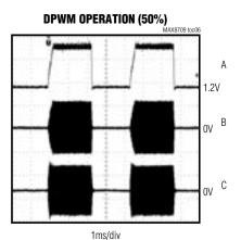
A: V<sub>CCV</sub>, 200mV/div B: V<sub>IFB</sub>, 1V/div C: V<sub>VFB</sub>, 1V/div
