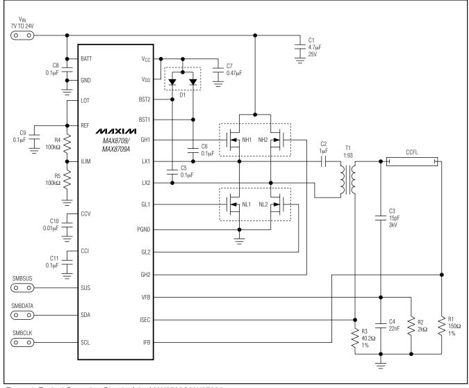
Figure 1. Typical Operating Circuit of the MAX8709/MAX8709A
