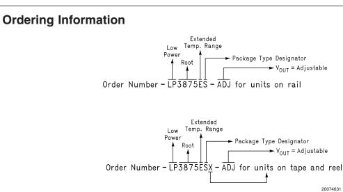
Package Type Designator is "T" for TO220 package, "S" for TO263 package, and "MP" for SOT-223 package.
