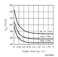
FIGURE 3.  $\theta_{JA}$  vs Copper(1 Ounce) Area for SOT-223 package
