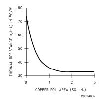
FIGURE 1.  $\theta_{JA}$  vs Copper (1 Ounce) Area for TO-263 package
