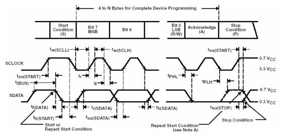
Figure 1. Timing Diagram, Serial Control Interface
