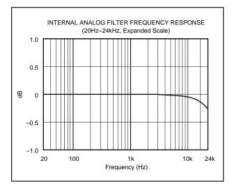
FIGURE 7. Low Pass Filter Frequency Response.
