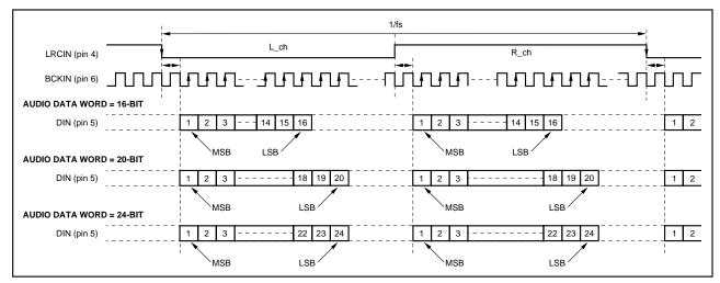
FIGURE 2. "I<sup>2</sup>S" Data Input Timing.
