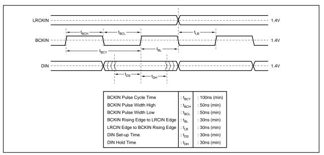
FIGURE 3. Audio Data Input Timing.
