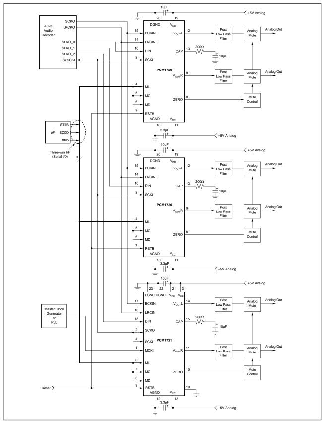
FIGURE 13. Connection Diagram for a 6-Channel AC-3 Application.
