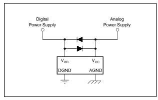
FIGURE 10. Latch-up Prevention Circuit.
