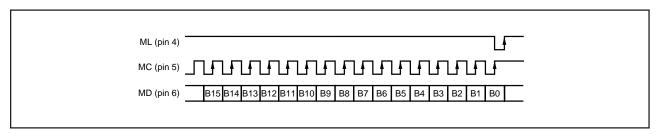
FIGURE 5. Serial Interface Timing.
