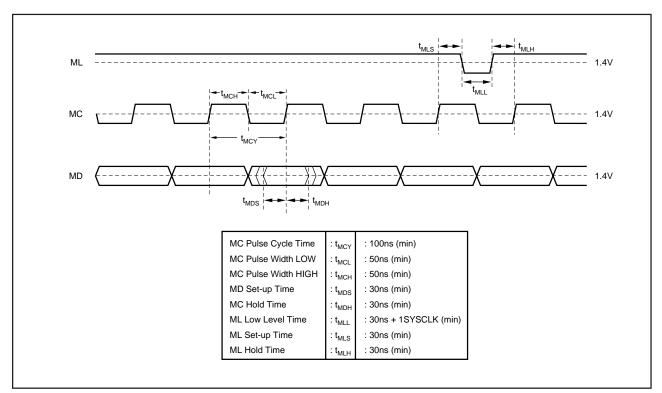
FIGURE 6. Program Register Input Timing.
