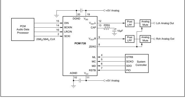
FIGURE 4. Typical Connection Diagram.
