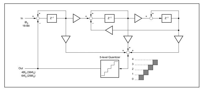
FIGURE 11. 5-Level  $\Delta\Sigma$  Modulator Block Diagram.
