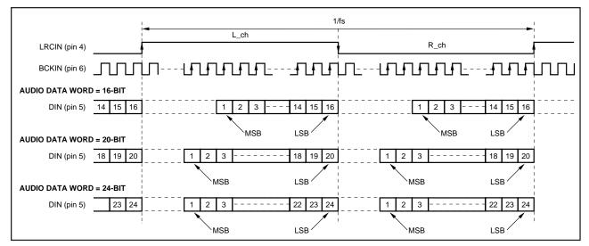
FIGURE 1. "Normal" Data Input Timing.
