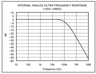
FIGURE 8. Low Pass Filter Wideband Frequency Response.
