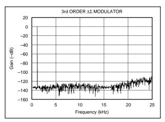
FIGURE 12. Quantization Noise Spectrum.
