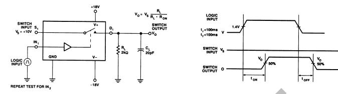
Switching Time Test Circuit
