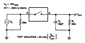
"OFF" Isolation Test Circuit
