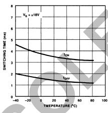
SSM2412 Switching Time vs. Temperature
