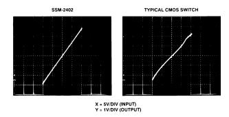
Figure 3. Comparison of the SSM2402 and Typical CMOS Switch for Distortion
