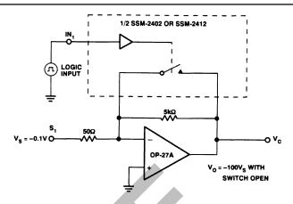
T<sub>ON</sub>/T<sub>OFF</sub> Switching Response Test Circuit
