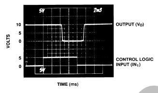
SSM 2412 T<sub>ON</sub>/T<sub>OFF</sub> Switching Response
