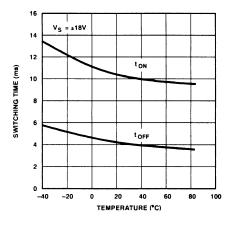
SSM2402 Switching Time vs. Temperature
