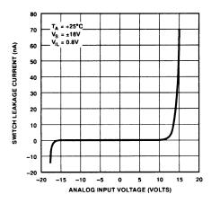
Leakage Current vs. Analog Voltage
