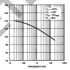
Channel Separation vs. Frequency
