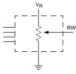
3-terminal Potentiometer; Variable Voltage Divider
