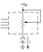
2-terminal Variable Resistor; Variable Current
