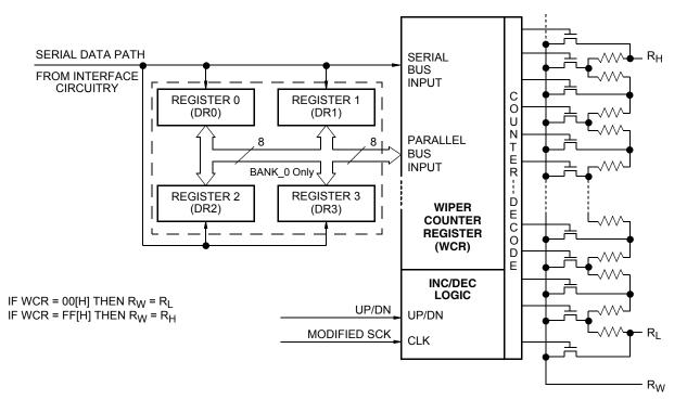
FIGURE 1. DETAILED POTENTIOMETER BLOCK DIAGRAM
