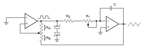
$<sup>\</sup>begin{array}{l} \mbox{Frequency} \propto R_1,\,R_2,\,C \\ \mbox{Amplitude} \propto R_A,\,R_B \end{array}$
