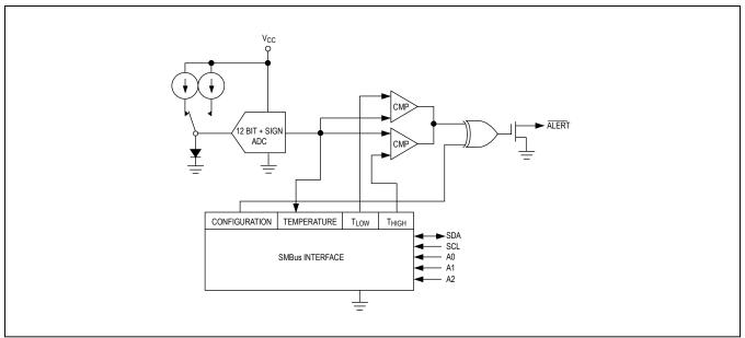
Figure 6. MAX6634 Functional Diagram
