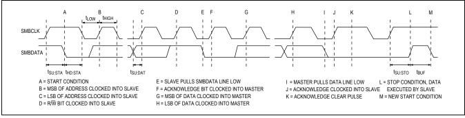
Figure 3. SMBus Read Timing Diagram
