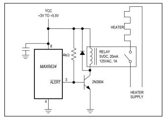
Figure 10. Simple Thermostat
