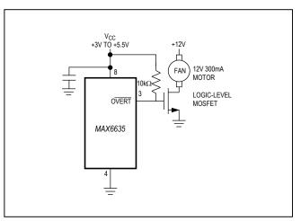
Figure 11. Fan Controller
