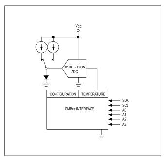
Figure 5. MAX6633 Functional Diagram
