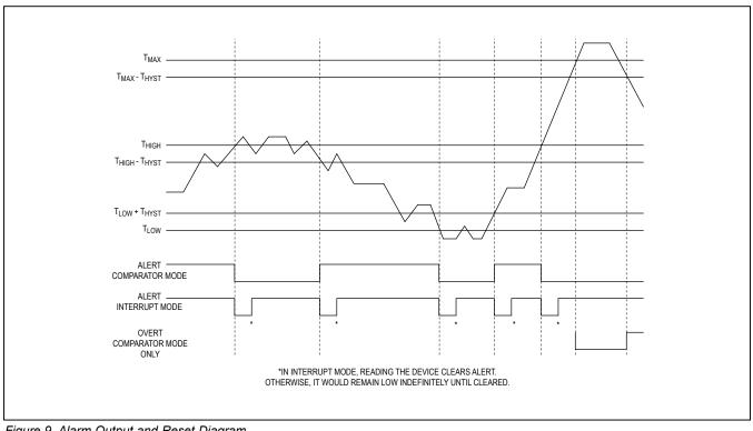
Figure 9. Alarm Output and Reset Diagram
