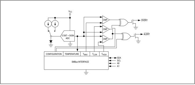
Figure 7. MAX6635 Functional Diagram
