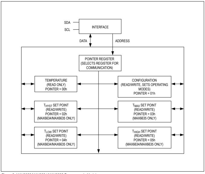
Figure 8. MAX6633/MAX6634/MAX6635 Programmer's Model
