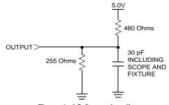
Figure 1: AC Output Loading
