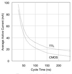
Figure 2: I<sub>CC</sub> (max) Reads
