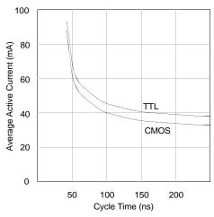
Figure 3: I<sub>CC</sub> (max) Writes
