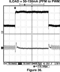
Buck 2 Load Transient Response VIN = 4.2V, VOUT = 3.3V ILOAD = 50-150mA (PFM to PWM)
