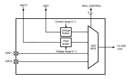
The source selection and the access to the conversion results are established through the I<sup>2</sup>C linked control registers: ADCC and ADCD as described below:
