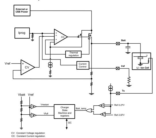
The charger module is a linear charger with constant current pre-qualification, constant current ("CC") full-rate charging and constant voltage ("CV") charging. CC and CV regulation is performed using an internal Power FET Q2 with reverse current blocking. The termination voltage is controlled to within ±0.35% at room temperature.
