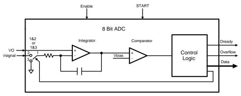
The A/D converter multiplexes 4 different sources:
