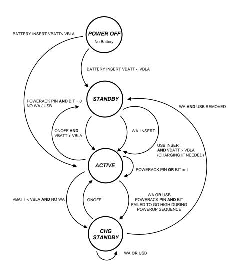
Figure 53. Operating Mode State Diagram
