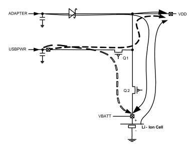
The current provided by the external adapter power or USB power, when inserted, first supplies the system load; the remainder is used for charging.
