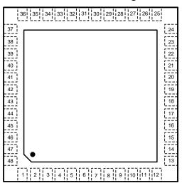
Figure 1. 48 WQFN Package (Top View) Package Number NJV0048A
