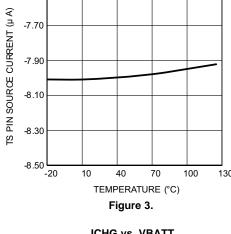
TS Pin Current vs. Temperature
