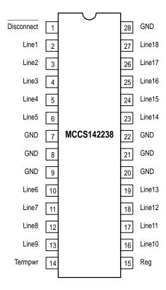
Figure 1. 28-Lead Pinout (Top View)
