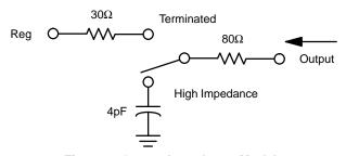
Figure 4. Output Impedance Model
