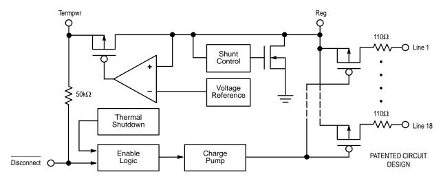
Figure 2. MCCS142238 Block Diagram
