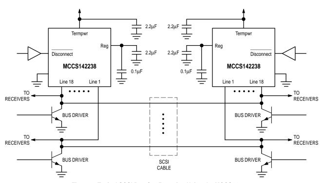
Figure 3. Typical SCSI Bus Configuration Using the MCCS142238
