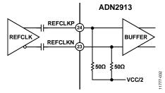
Figure 30. AC-Coupled, Differential REFCLKx Configuration
