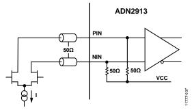
Figure 36. DC-Coupled Application, 0 dB EQ Input (Normal Mode)
