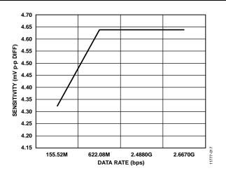
Figure 15. Sensitivities of SONET/SDH Data Rates (BER =  $10^{-10}$ )
