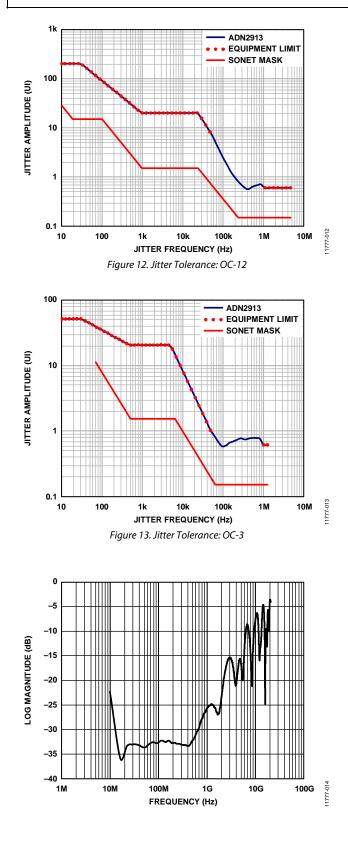
Figure 14. Typical S11 Spectrum Performance
