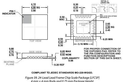
4 mm × 4 mm Body and 0.75 mm Package Height (CP-24-7) Dimensions shown in millimeters
