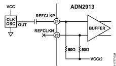
Figure 29. AC-Coupled, Single-Ended REFCLKx Configuration
