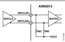
Figure 28. DC-Coupled, Differential REFCLKx Configuration
