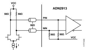
Figure 37. DC-Coupled Application, 0 dB EQ Input (Back Terminated Mode)
