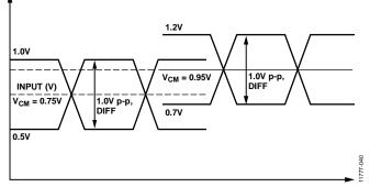
Figure 34. Maximum Allowed DC-Coupled Input Levels
