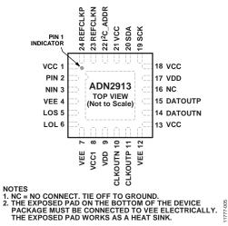
Figure 5. Pin Configuration
