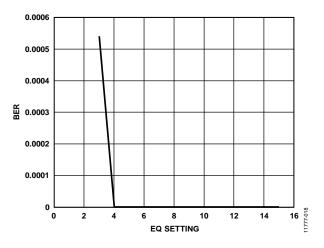
Figure 16. BER in Equalizer Mode vs. EQ Compensation at 8GFC (Measured with an 8GFC Signal of 400 mV p-p diff, on 15-Inch FR4 Traces, with Variant EQ Compensation, Including Adaptive EQ)
