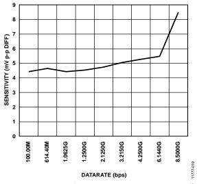
Figure 17. Sensitivities of non-SONET/SDH Data Rates (BER =  $10^{-12}$ )
