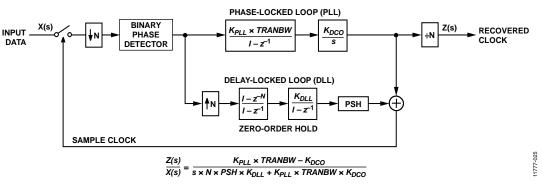
Figure 23. CDR Jitter Block Diagram
