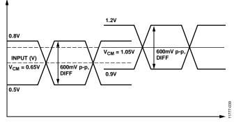
Figure 33. Minimum Allowed DC-Coupled Input Levels
