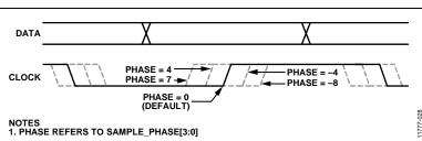
Figure 26. Data vs. Sampling Clock
