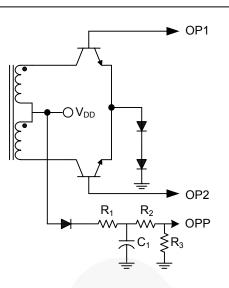
Figure 18. OPP Protection Circuit
