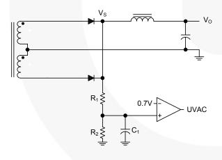
Figure 17. AC Detection Circuit
