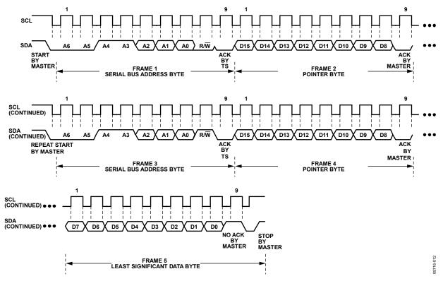
Figure 17. A Write to the Pointer Register Followed by a Repeat Start and an Immediate Data-Word Read
