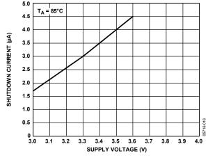
Figure 8. Shutdown Current vs. Supply Voltage
