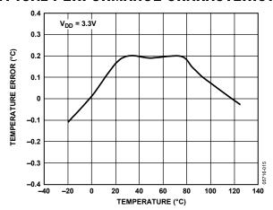
Figure 5. Temperature Accuracy
