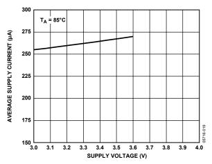
Figure 7. Supply Current vs. Supply Voltage
