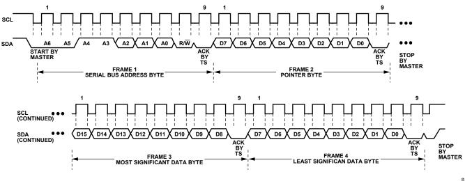
Figure 14. Writing to the Address Pointer Register, Followed by Two Bytes of Data
