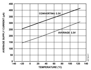
Figure 6. Supply Current vs. Temperature
