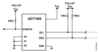
Figure 13. Typical SMBus/I<sup>2</sup>C Interface Connection
