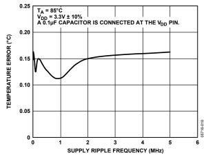
Figure 9. Temperature Accuracy vs. Supply Ripple Frequency
