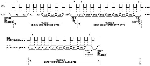
Figure 16. Reading Back Data from the Register with the Preset Pointer
