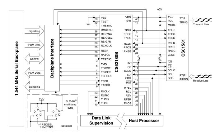
Figure 17. Typical System Connection
