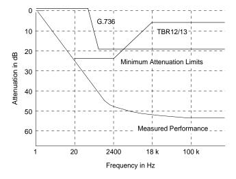
Figure 11. Typical Jitter Transfer Function - E1
