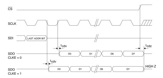
Figure 5. Serial Port Read Timing Diagram
