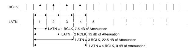
Figure 9. LATN Pulse Width encoding
