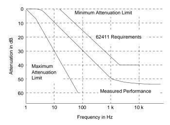
Figure 10. Typical Jitter Transfer Function - T1
