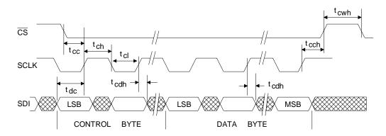
Figure 4. Serial Port Write Timing Diagram
