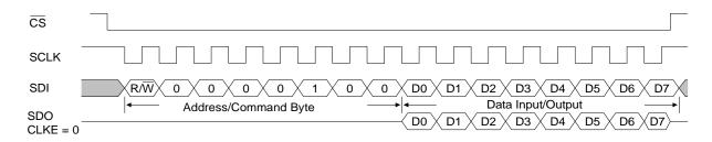
Figure 12. Input/Output Timing (showing address 0x10)
