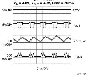
Typical Switching Waveform in Boost Mode (PWM Mode)
