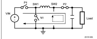
FIGURE 3. Simplified Circuit for Buck Operation
