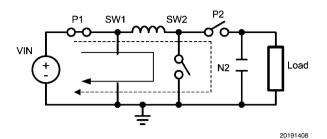
FIGURE 4. Simplified Circuit for Boost Operation
