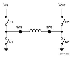
FIGURE 2. Simplified Diagram of Switches
