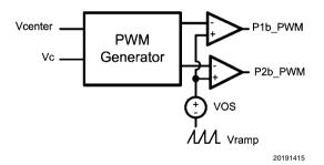
FIGURE 5. PWM Generator Block Diagram
