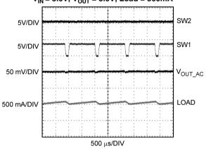
Typical Switching Waveformt in Boost Mode (PFM Mode)
