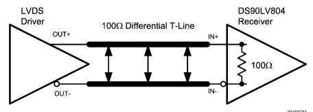
Typical LVDS Driver DC-Coupled Interface to DS90LV804 Input
