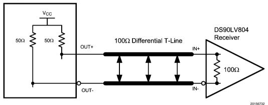
Typical CML Driver DC-Coupled Interface to DS90LV804 Input
