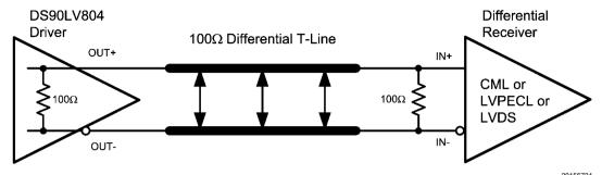
Typical DS90LV804 Output DC-Coupled Interface to an LVDS, CML or LVPECL Receiver
