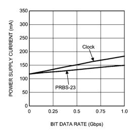
Dynamic power supply current was measured while running a clock or PRBS 223-1 pattern with all 4 channels active.  $V_{CC}=3.3V$ ,  $T_A=+25^{\circ}C$ ,  $V_{ID}=0.5V$ ,  $V_{CM}=1.2V$
